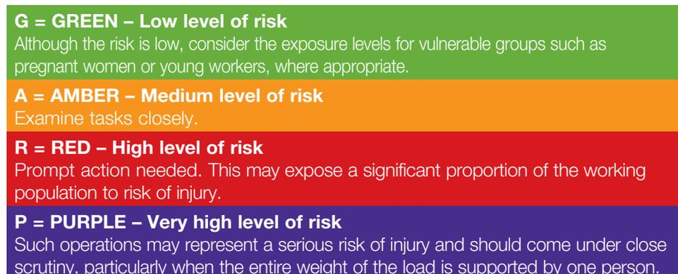
**Figure 23** The MAC colour bands showing the 'traffic light' approach
